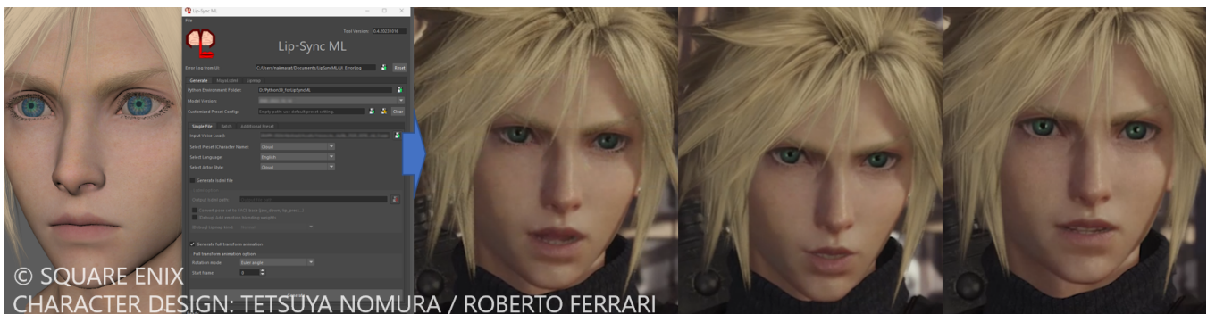
Figure 1: Lip-sync animation generated by Lip-Sync ML. From the voice audio of a character, the tool (left) can generate the animation, and it can be played in a game engine (right.)
