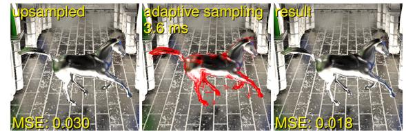
**Figure 16:** Adaptive recomputation for the spatio-temporal upsampled image (Fig. 15) evaluating low-weight pixels. The horse is a dynamic object. A threshold 0.25 is used for resampling in this experiment.
