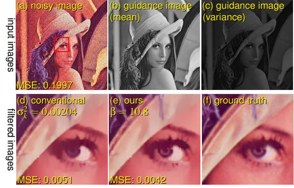
**Figure 3:** Distribution-aware filtering with Gaussian functions represented with guidance images (b) and (c). The noise of the input image (a) is proportional to the variance (c). Our filtering (e) preserves the edges of the eye, while cross bilateral filtering (d) does not. Both  $\sigma_k^2$  and  $\beta$  are optimal for this image.
